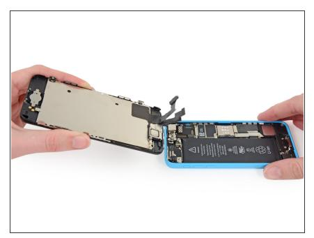
Remove the front panel assembly from the rear case.
