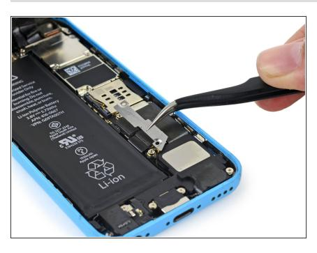
Remove the metal battery connector bracket from the iPhone.
