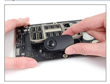
• Remove the speaker from the IO board.
