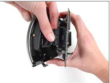
• Squeeze and pull the audio jack ribbon cable connector from the IO board.
