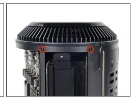
• Remove five 5.1 mm T10 Torx screws from around the outer perimeter of the fan assembly.
