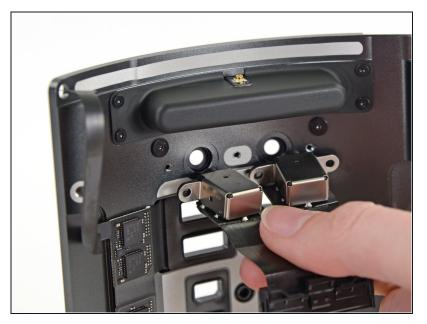
Carefully pull and remove the audio jacks straight away from the IO panel.
