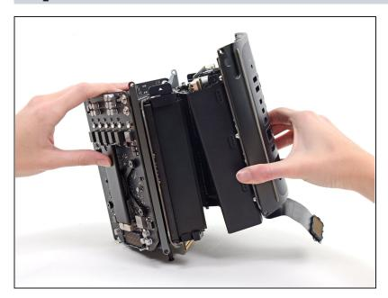
• Remove the power supply assembly from the Mac Pro.
