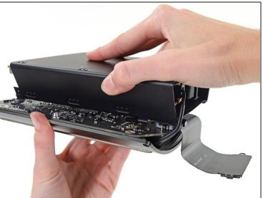
• Gently shift the power supply to free the AC power inlet cable out of its plastic clip.
