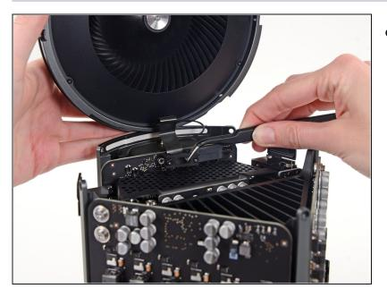
Use a pair of <u>tweezers</u> to pull the fan cable bracket away from the fan assembly.
