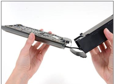
• Flip the power supply back to expose the AC power inlet cable.
