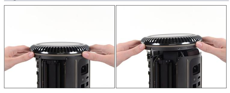
• Carefully lift the lower case up and remove it from the Mac Pro.
