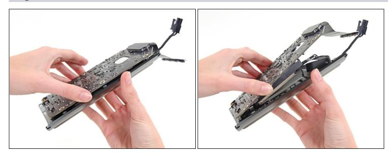
• Lift the IO board up from the IO shield from the end with the AC plug.
