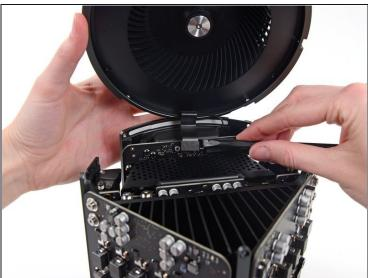
• Use the flat end of a spudger to disconnect the fan assembly ribbon cable from the IO board.
