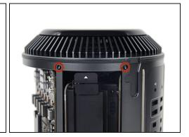
• Remove five 5.1 mm T10 Torx screws from around the outer perimeter of the fan assembly.
