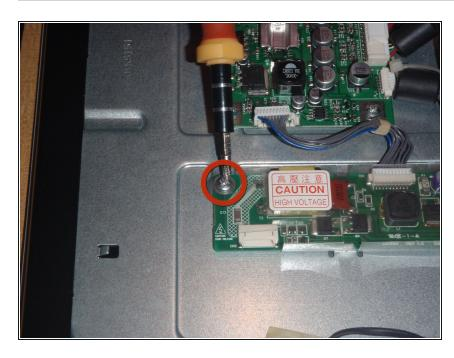
Remove the top philips head screws holding the board to the monitor with #2 philips head screwdriver.
