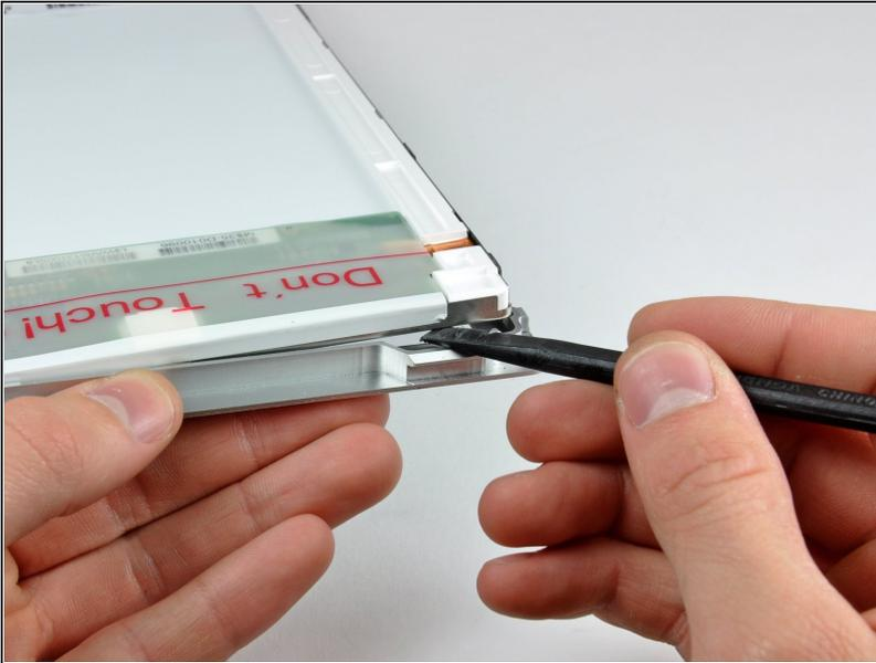
ⓘ The next few steps will require you to separate the LCD from the adhesive applied to the upper and lower edges of the front bezel. A heat gun may be helpful to soften the adhesive to prevent damaging the LCD panel during removal.
