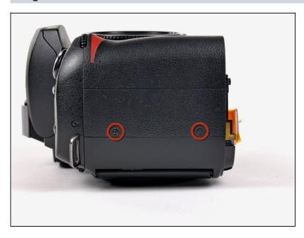
Remove the two Phillips screws securing the grip side of the rear cover to the D70.
