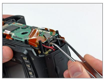
Use a pair of tweezers to pull the USB connector bracket away from the edge of the memory compression board.
