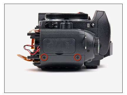
Remove the two Phillips screws securing the DC-In side of the rear cover to the D70.
