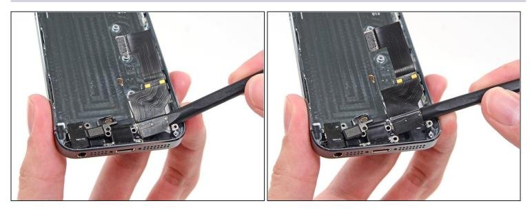
• Continue to detach the lightning cable assembly by sliding the spudger under the port components.
