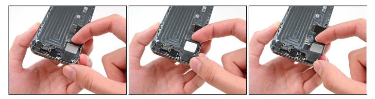
• Remove the speaker by lifting it up and out of the rear case.
