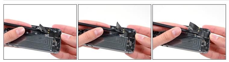
• Slide the flat end of a spudger under the right-hand side of the lightning connector cable assembly to free it from the rear case.
