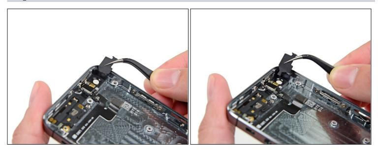
• Use tweezers to pull the rubber rear-facing camera cover out of its slot in the rear case.
