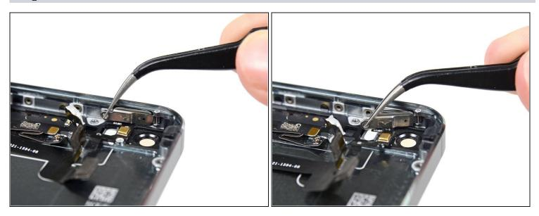
• Use a set of tweezers to swing the power/sleep button bracket away from the case.
