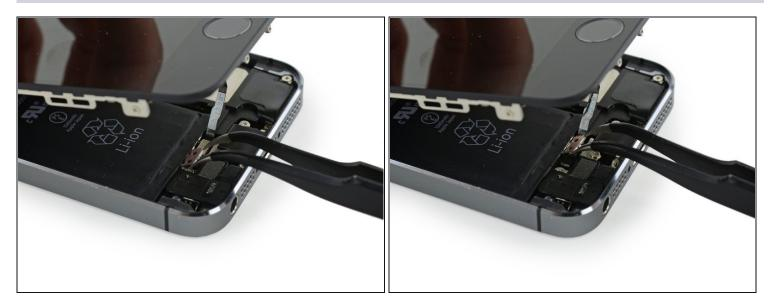
During reassembly, you will need to reinstall the Touch ID cable bracket. The top of the bracket needs to slide between the battery and Touch ID cable connector, in front of the metal tab. The bottom must latch down over the connector.
