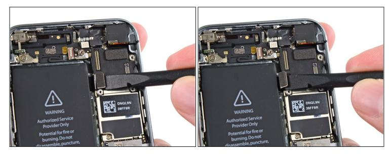
• Use a spudger to gently pry the button assembly cable up from its socket on the logic board.
