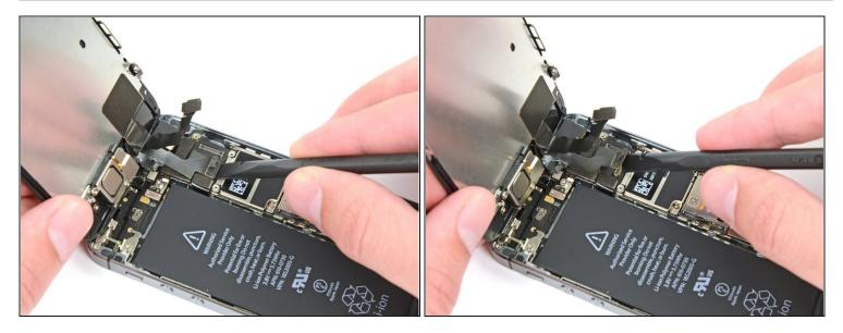
A Make sure the battery is disconnected before you disconnect or reconnect the cable in this step.
