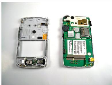
Gently lift and remove the back casing.
