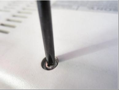
• Flip over the PlayStation and remove the six screws from the bottom.
