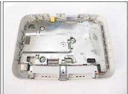
Disconnect the cables from the PSone's board.
