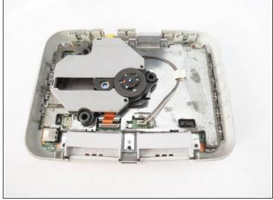
Lift up and remove the upper case.
