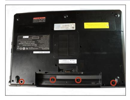
• Remove the screws and flip it back.
