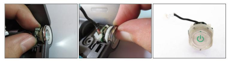
• While pulling the button upwards and towards the left (left fingers), push the button inwards (right fingers) at the same time to remove it from its place.
