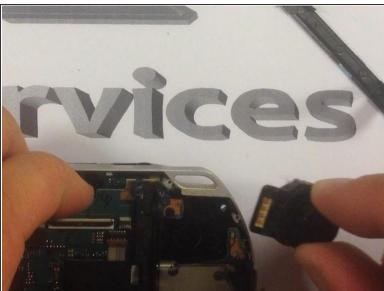
Slightly lift the board and remove the joystick!
