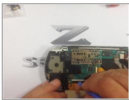
Be careful while removing the screen! Release the cables for screen and "volume-start-home keys"!
