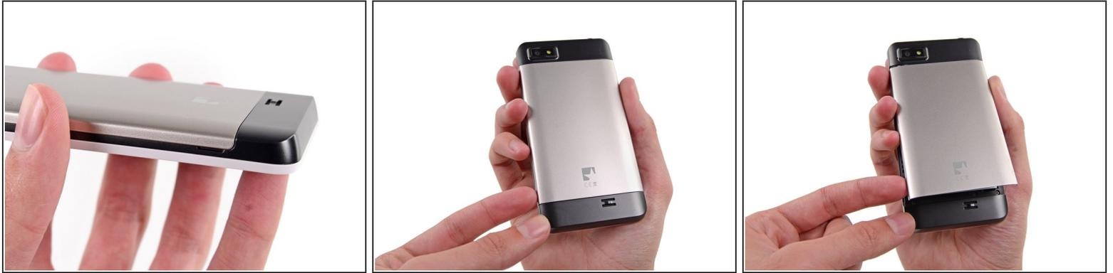
**i** There is a small indentation in the side of the phone near the bottom of the back cover.
