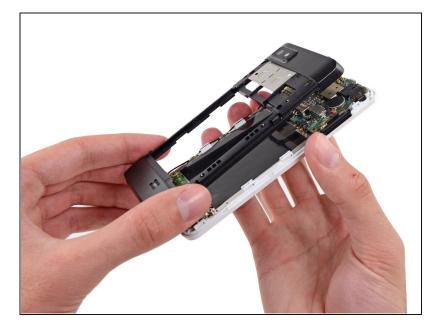
Separate any remaining clips and remove the midframe from the phone.
