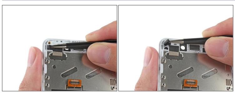
• Remove the rubber guide from the recess near the front facing camera hole.
