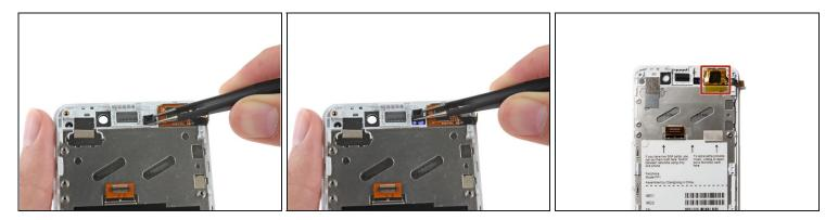
• Remove the rubber guide to the right of the earpiece speaker recess.
