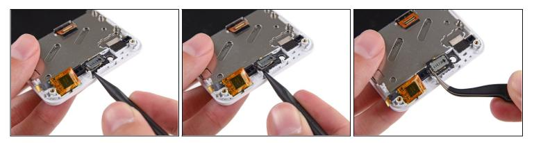
(i) The earpiece speaker is held to the back of the display assembly with some mild adhesive.
