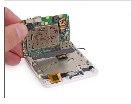
Remove the motherboard from the display assembly.
