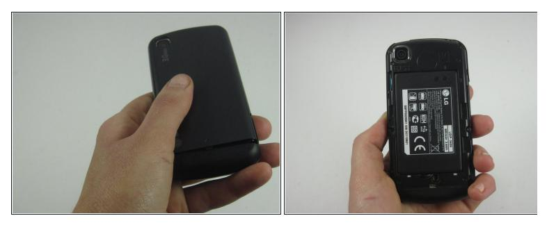
• Push up on the back cover to slide it off and reveal the battery underneath.
