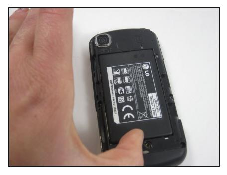
• Use your nail or a spudger to gently pry the battery out from the bottom of the phone.
