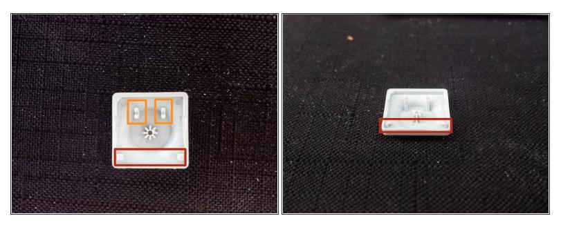
The red area is the back of the key and the orange tabs are where the key connects into the previously labeled orange scissor clips.
