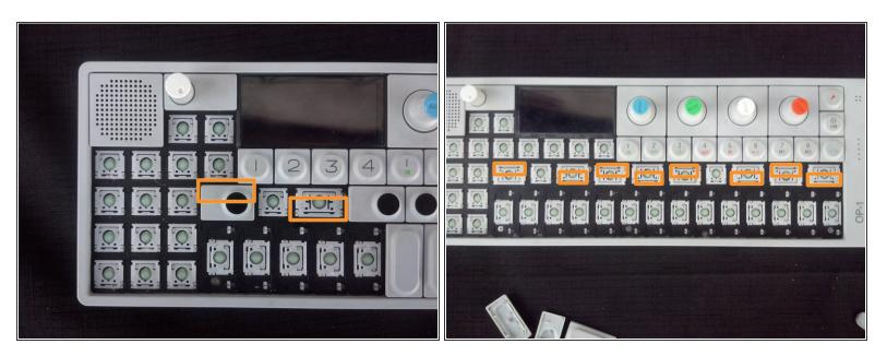
• Removing the rest from here is pretty straight forward except for one part. The black piano keys alternate tab removal access points. They are labeled for your enjoyment
