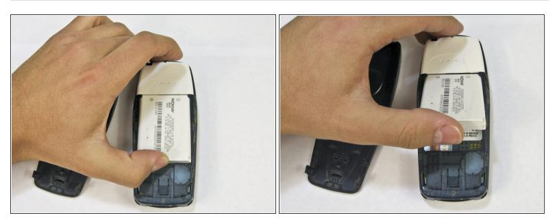
• Lift the battery near the bottom and pry up.
