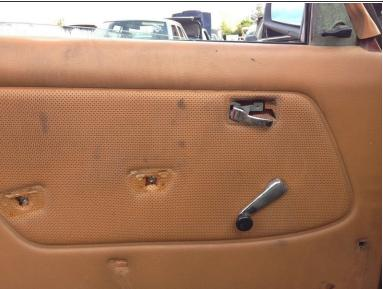
Remove the two screws under the armrest. These are often extremely overtightened and may be hard to remove.
