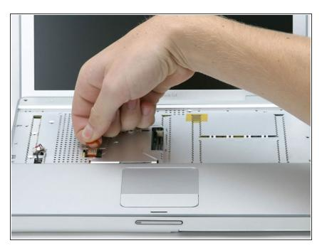
• Use the orange plastic loop to disconnect the trackpad cable.
