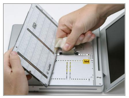
Grasp the keyboard connector ribbon near the connector and disconnect it from the logic board.
