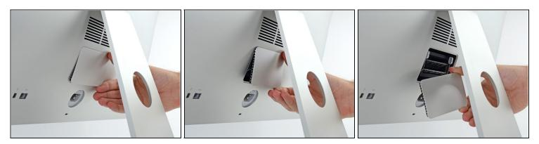
• Pull the RAM access door off the back of the iMac.
