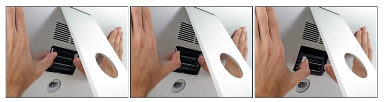
(i) The RAM tray is locked into its upright position with two grey tabs.
