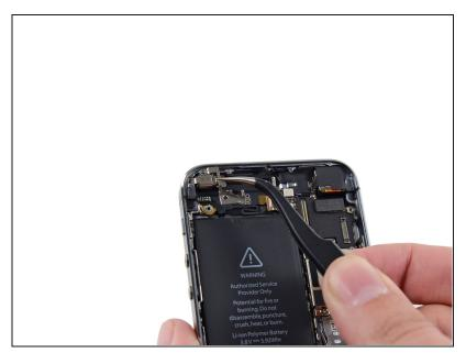
• With a set of <u>tweezers</u>, remove the vibrator bracket.
