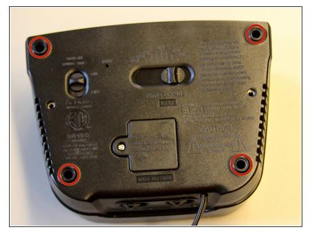
Flip device upside down and remove the 4 foam pads at each corner.
