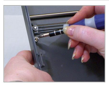
Remove the screw holding the tension spring in place.
