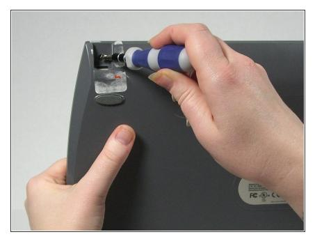
On the bottom of the scanner, remove the screw at the top left side.
