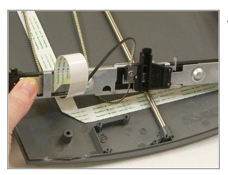
Loosen the belt enough to turn over the sensor bar.
