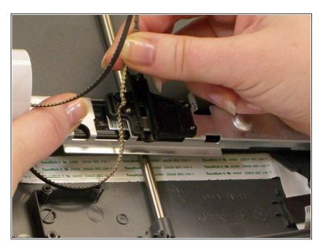
Carefully lift the belt out of the groove in the sensor bar to remove.
