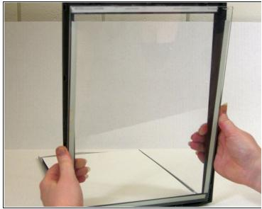
With consistent pressure on the glass, move your fingers down the sides until the glass is no longer stuck to the double-sided tape.
