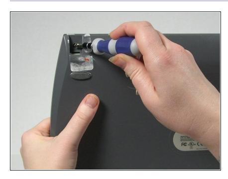
On the bottom of the scanner, remove the screw at the top left side.
