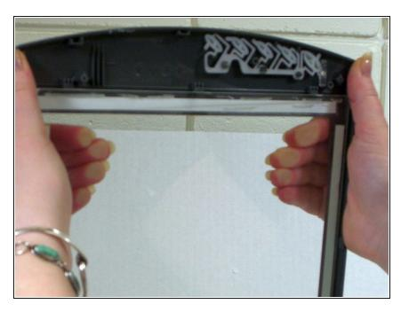
Apply even pressure against the back of the glass while securing the plastic frame in place.
