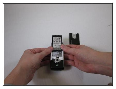
• Slide the battery upward to remove.
