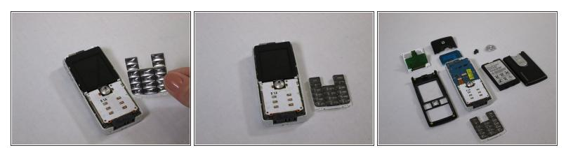
• Remove the keyboard by slowly pulling it away from the circuit board.
