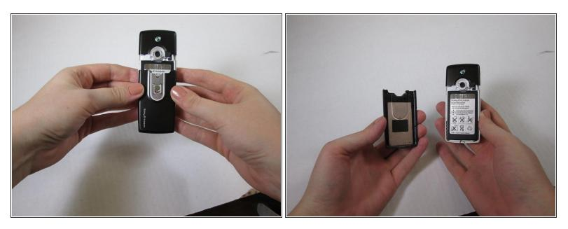
Slide the protective panel on the backside of the phone downward and remove it entirely, revealing the battery underneath.
