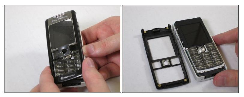
• Gently lift and remove the front panel of the phone after removing the screws.
