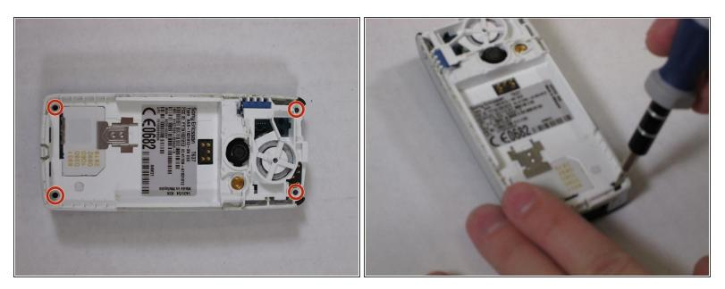
• Remove the four screws located at each corner of the device.
