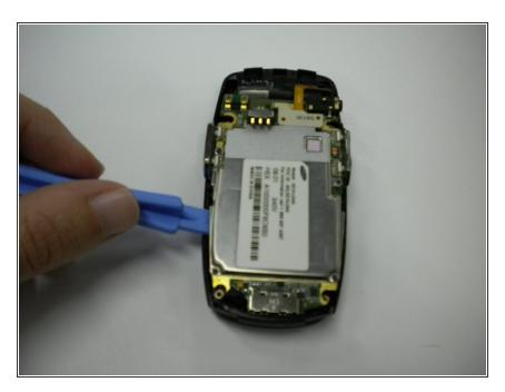
• Use spudger to pry logic board from the casing.
