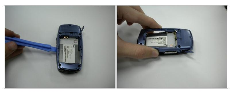
• Use a spudger to pry the back assembly off of the device.
