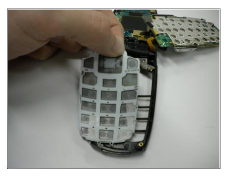
• Lift the number pad straight up from the casing.
