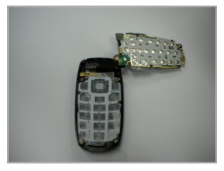
Rotate the logic board assembly out of the casing, being careful not to break VGA cable.
