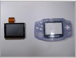
Use the spudger to lift the screen from the front panel. Place the spudger in the space directly left of the D-pad.
