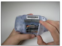
• Take the battery cover off by releasing the locking tab and hinging the cover away. Remove the batteries inside the cover
