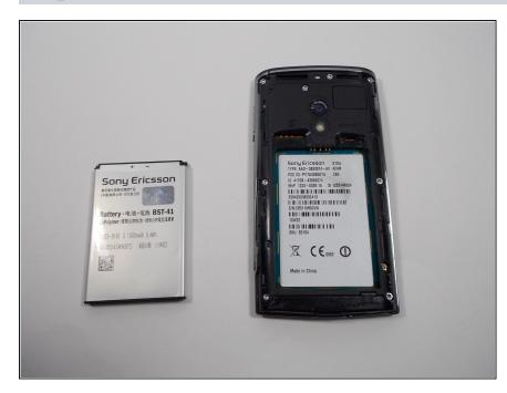
The first step in accessing the audio and/or camera buttons is to remove the back case of the phone and then the battery
