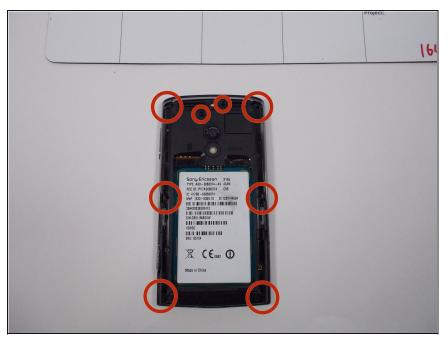
• Use a Torx T6 screwdriver to remove eight 5 mm screws on the back case.
