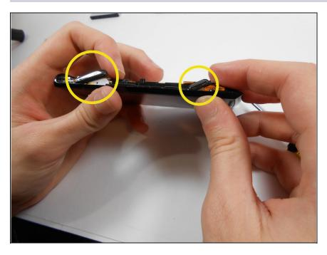
The volume button (left) and the camera button (right) lift right out of the phone as shown in the picture. From here you can clean them or replace them.
