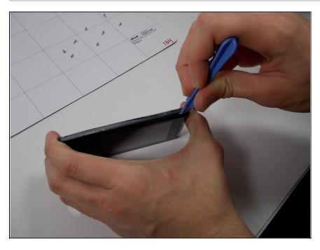
Using an opening case, (a guitar pick works as well), start on the bottom right side of the phone and undo the clips located at the interior sides.
