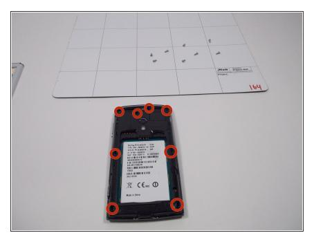
Remove the eight 5mm T6 screws from the back of the phone.
