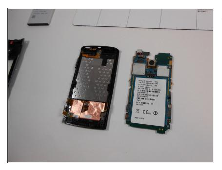
Remove the logic board and put it to the side.
