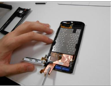
Using a flat head screw driver, disconnect the glue holding the left ribbon cable to the phone. Pull
