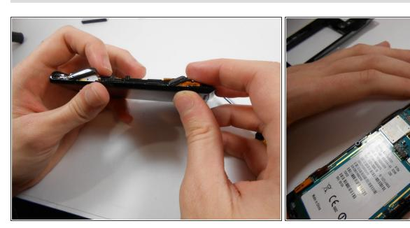
Remove the volume and camera buttons. Using your fingers or a screwdriver, pull off the black plastic piece on the very top of the phone.
