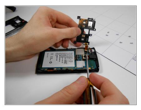
Using a flat head screwdriver, flip the chip to the left and remove the ribbon cable.
