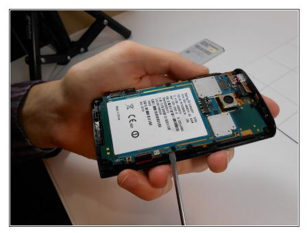
Gently insert a flat head screw driver under the logic board and pry to remove it from the phone casing.
