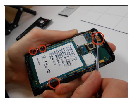
Using a flat head screw driver, undo the ribbon cables connected to the phone.
