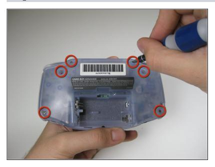
Remove the six back panel screws using a Y1 screw driver.
