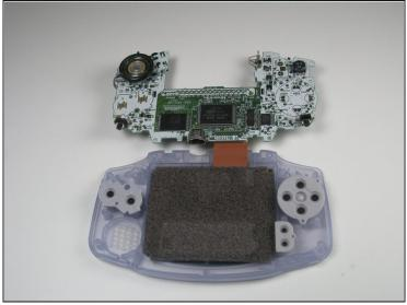
• Pull circuit board away from the front panel by pulling up at the bottom of the circuit board, keeping the top ribbon still connected.
