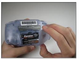
• Remove the back battery cover by pinching down on the tab and pulling outward.
