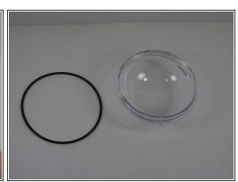
Using a plastic spudger, lift the o-ring from the lid
