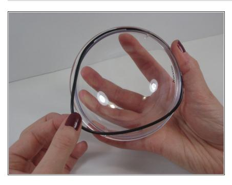
Gently stretch the new O-ring and place it in position on the clear cover. Make sure it is flush with the flange and not interfering with the locking threads
