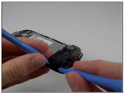
• Use a plastic opening tool to remove each area holding the parts together.
