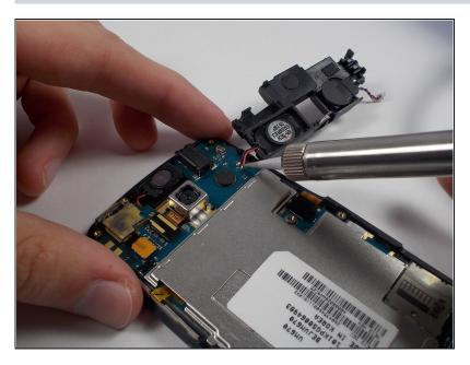
Solder off the antenna, and solder on the new one. The antenna is now replaced.
