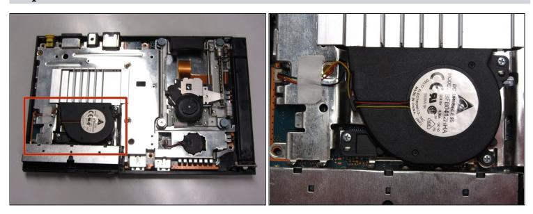
• Locate the fan at the front, left section of the unit.
