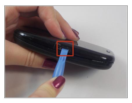
After screw is removed take the plastic opening tool and apply slight pressure to even out bends in the metal
