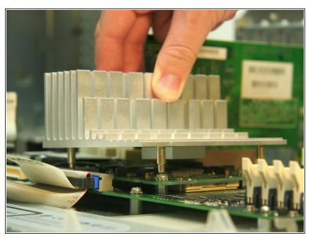
• Remove the heat sink by pulling upwards, off of the logic board.
