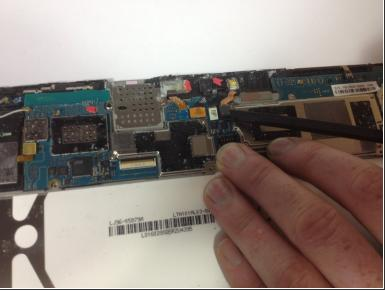
Use the spudger to pry up on the white connection of the rear camera wire.
