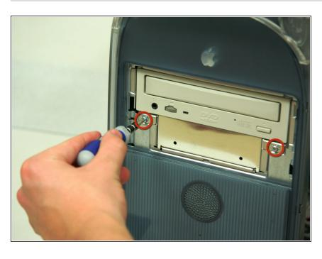
Remove the two screws on the front of the drive with the Phillips #1 screwdriver.
