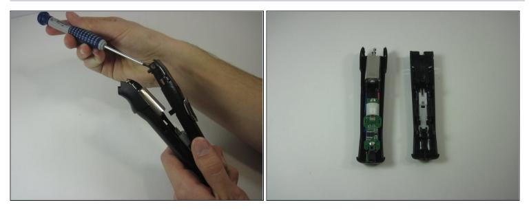
• Pry open the plastic cover into two separate pieces. The plastic is very durable so don't worry about breaking it upon prying it open.
