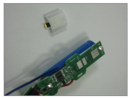
• Remove the white plastic cover over the chip set allowing the battery to be taken off.
