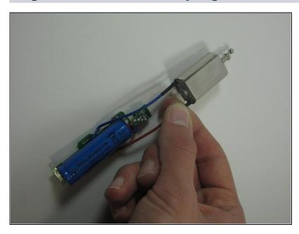
Remove the chip set, motor and battery from the plastic body. This photo shows the motor and wires connecting it to the battery.
