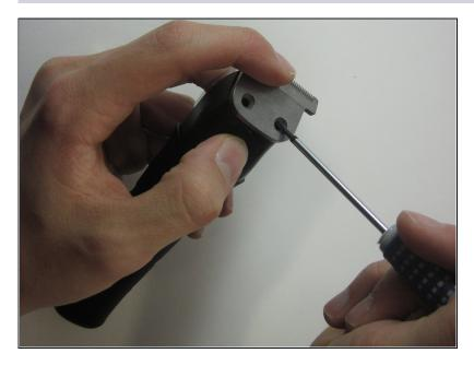
• Remove the screws from the top to take the metal piece and plastic part off.
