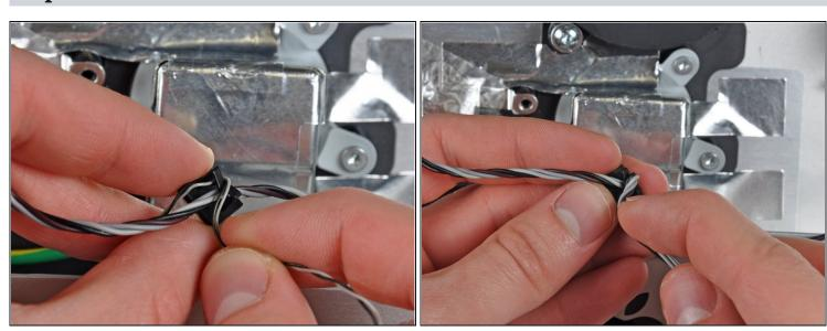
• Carefully remove the left speaker and ambient temperature sensor cables from the CPU fan cable retainer.
