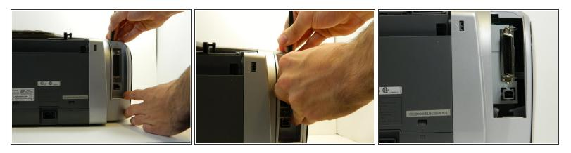
• Wedge the flat end of the spudger between the top of the "Parallel" cover and the right panel, and gently pry the upper edge cover away. Completely remove the cover by hand if necessary. The Parallel and USB ports should be exposed.
