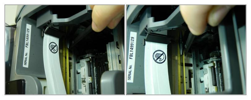
• Use the flat end of the spudger to push the white button next to the ink cartridge carrier.
