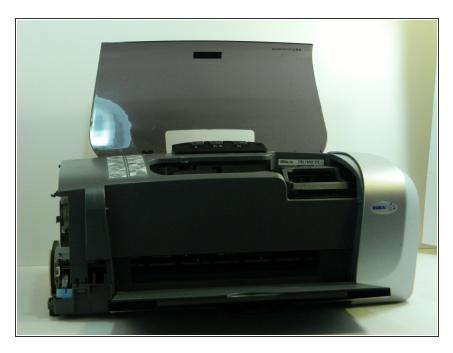
• Gently push the panel to the right to separate it from the printer.
