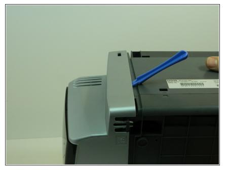
Wedge a blue plastic separator between the plastic housing and the rest of the right panel and push the panel out from the inside to free it.
