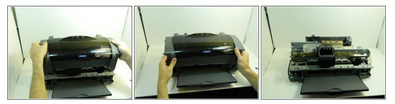
• Gently pull the plastic housing upward to remove the back panel and reveal the inner components of the printer.
