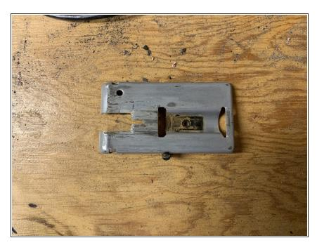
After removing M4 screw, remove the base plate and place to the side.
