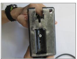
Orient your saw so that the blade is pointing in the opposite direction of your body. Ensure that the screws circled are visible and pointing skyward. This will be the standard position of the Jigsaw for the duration of this guide.
