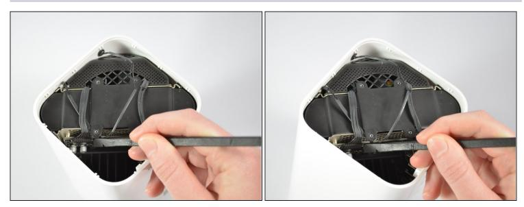
A Four black internal wires, three thin and one thick, are connected to the logic board: three by small end clips and one by a larger end clip. Handle the clips gently; they break easily.
