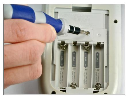
Using the Phillips #00 Screwdriver, unscrew the 15 mm screw holding the backup battery cover, located above the main battery area.
