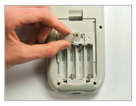
• Grab the plate and lift gently upward, to remove the backup battery cover.
