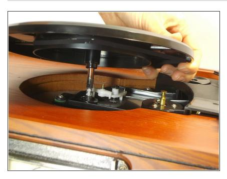
Using your thumb as a guide, place the platter back onto the motor so that the peg holding the drive-belt wraps around the outside of the brass motor post.
