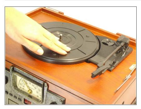
Secure the platter all the way down and spin the platter clockwise until you hear a pop and feel resistance from the drive-belt catching.
