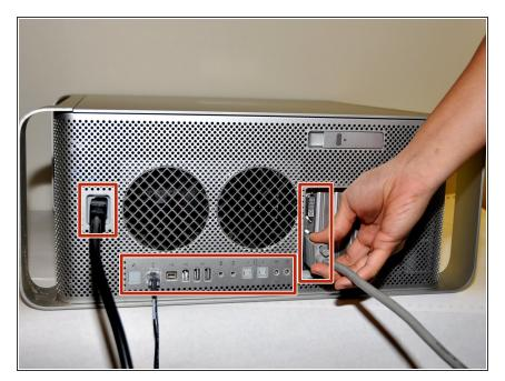
Remove all the cables, including the power cables before opening the unit.
