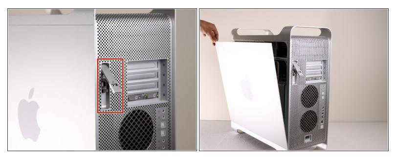
• Lift the tab to unlock the side panel.
