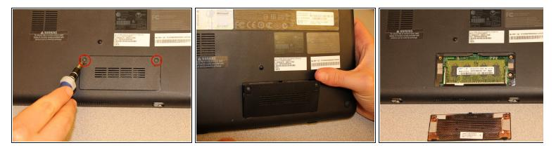
• Flip the netbook over so you are looking at the bottom, and locate the two screws that hold the memory card cover.
