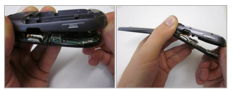
Lift the back cover starting at the bottom of the phone.
